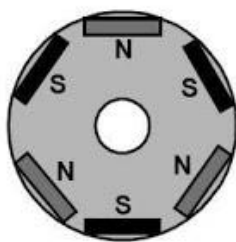
Circular core with rectangular magnets embedded in the rotor
