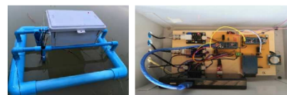
Fig. 2. The picture of buoys is used as data collector instruments. The buoys are used as data collectors near tilapia fish cages in the dam. The picture also identifies the IoT instruments in each buoy
