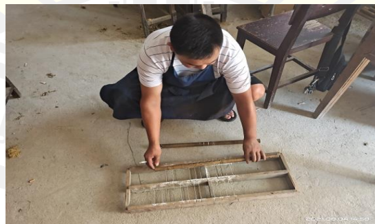
Figure 22 Locate the sound holes by using molds
