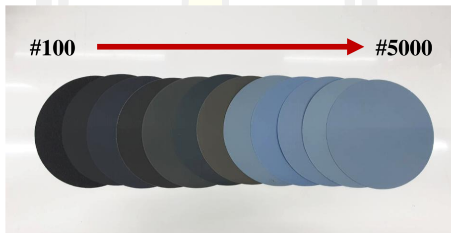
Figure 3.18 The SiC sandpapers with grit sizes of 100, 200, 600, 800, 1000, 1500, 2000, 2500, 3000, 4000, and 5000.
