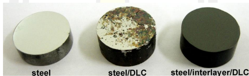
Figure 2.5 Surface characteristics of (a) the AISI 4140 steel polished, (b) DLC without interlayer on steel, and (c) DLC with a-SiC x :H adhesion interlayer on steel [74].
