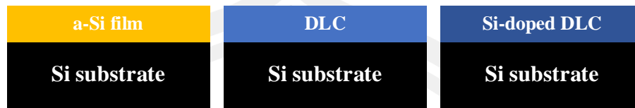
Figure 5.1 The schematic model of the a-Si interlayer, the DLC film and the Si-doped DLC film on silicon substrate (not to scale).
