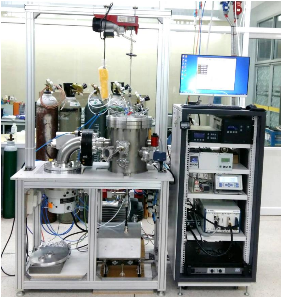
Figure 3.2 A photo of a hybrid RF-PECVD/MS system used for a-C:H with silicon-based interlayer deposition.
