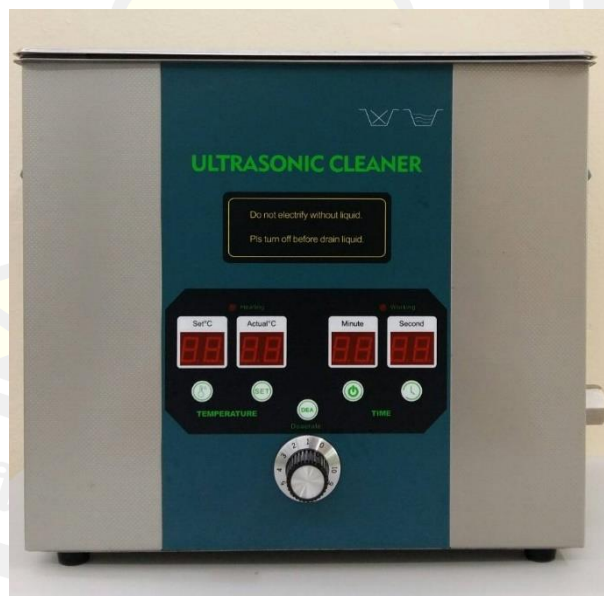
Figure 3.14 A photo of the ultrasonic cleaner for substrate cleaning.
