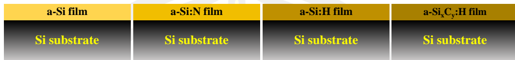
Figure 4.1 Schematic model of four silicon-based interlayers on a silicon substrate (not to scale).
