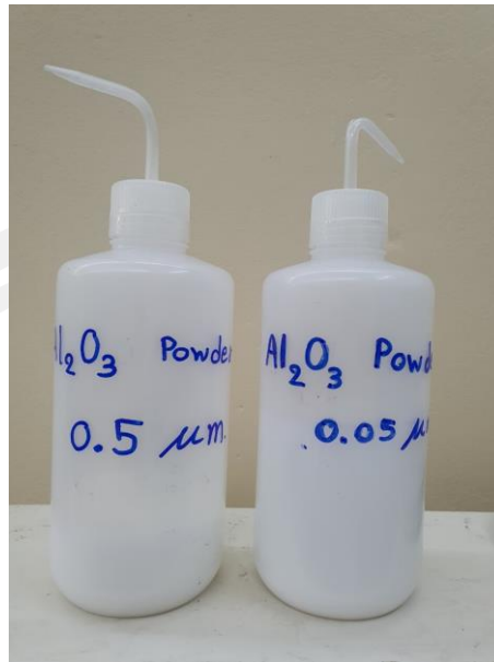
Figure 3.19 The alumina powder with particle size of 0.5 \mu\text{m} and 0.05 \mu\text{m} used for suspension in DI water.
