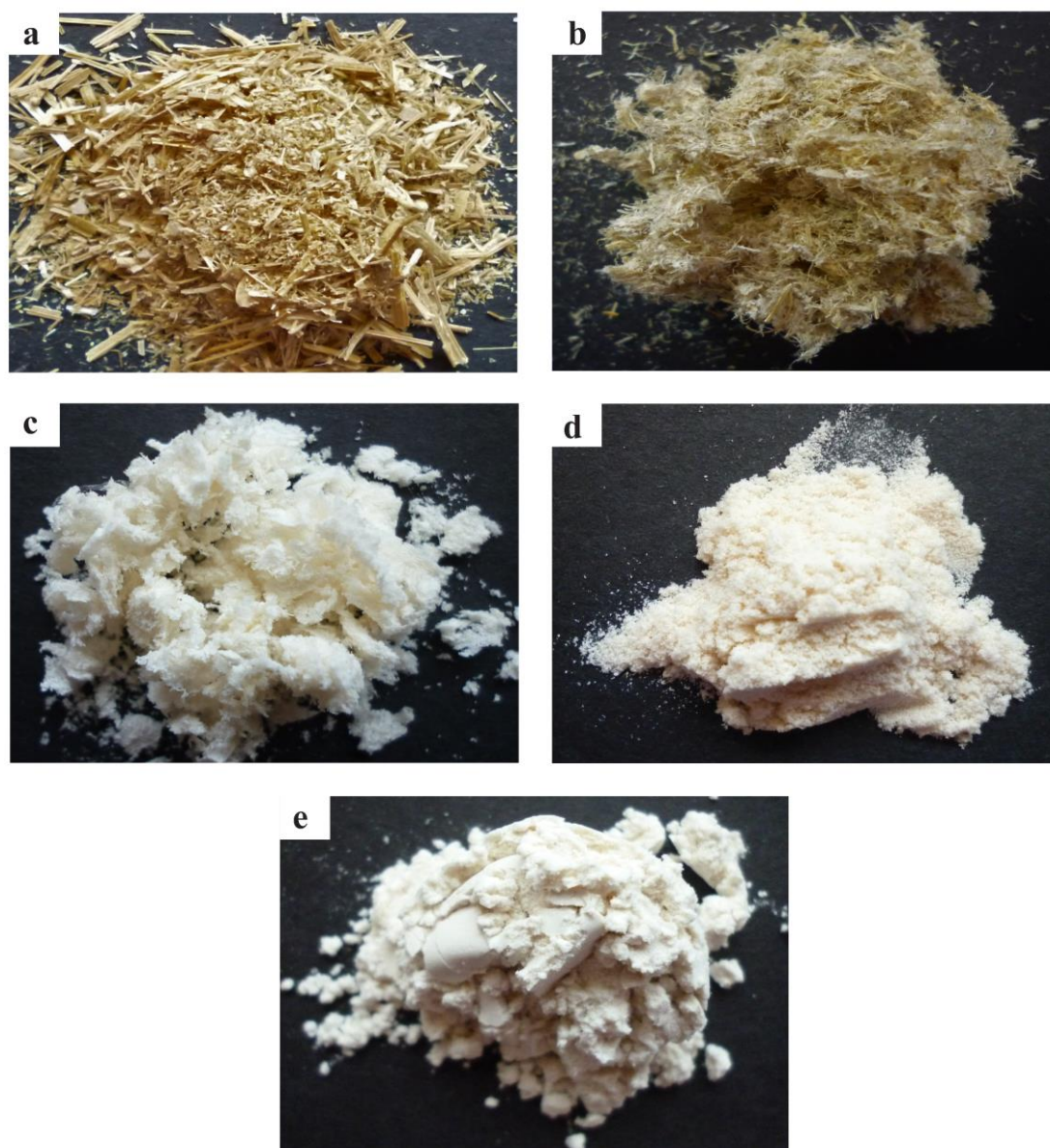
Figure 26 Physical appearances of rice straw (a), alkali-treated rice straw (b), bleached rice straw (c), NC (d) and modified NC (e)
