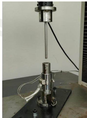
(20) Single pellet compressor
