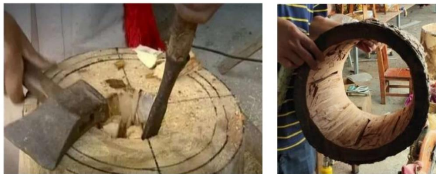
Figure 21 Cutting through shaded wood with a chisel.
