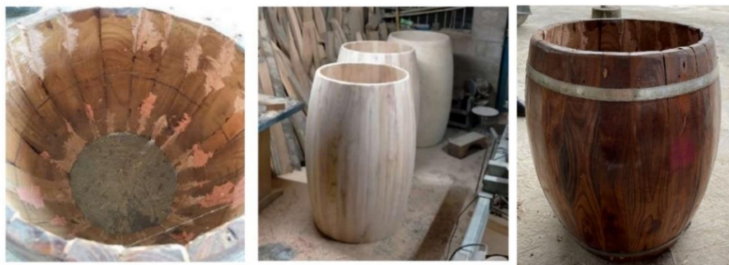
Figure 30 Bonding, polishing, painting, and installation of copper rings
