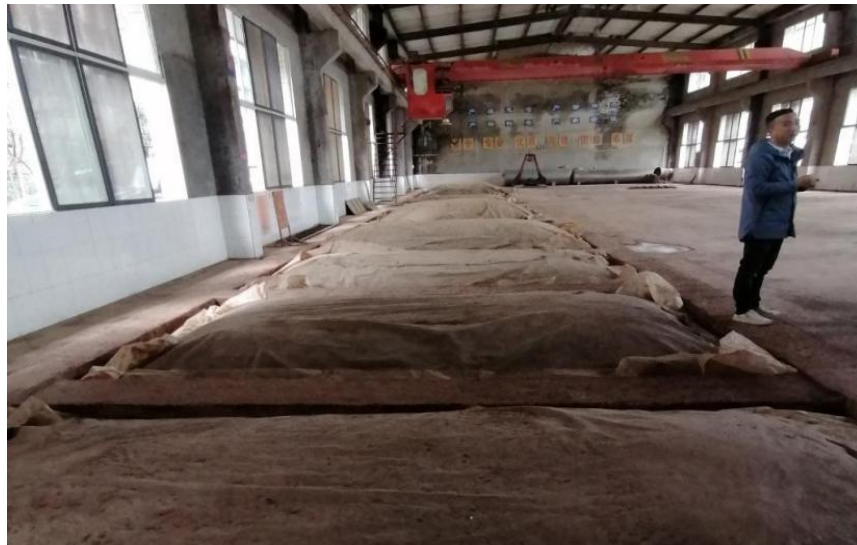
Figure 31 The difference between sauce-flavored Moutai liquor and other flavored liquors is that the pits of Maotai-flavored liquores are made of stones, and the pits should be sealed with local yellow mud, which is not breathable. Wet and closed, sprinkle water frequently to prevent dry cracks from entering the air.
