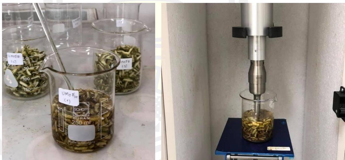
Figure 17 Ultrasonicated MOF at 20 kHz.
