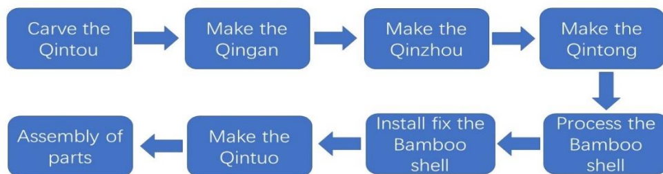
Figure 27. Flowchart of making Zhutonghu,
