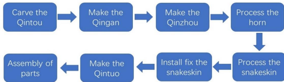
Figure 29. Flowchart of making Jiaohu.
