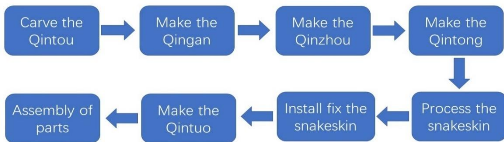
Figure 20. Flowchart of making Maguhu,
