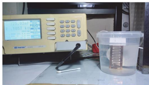
Fig.4. The measurement setup for IDC level sensor.
