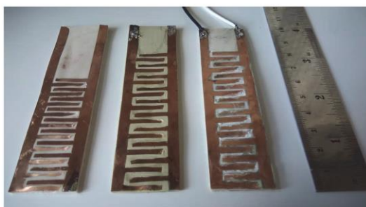
Fig.2. The fabricated the novel IDC level sensor with epoxy substrate .
