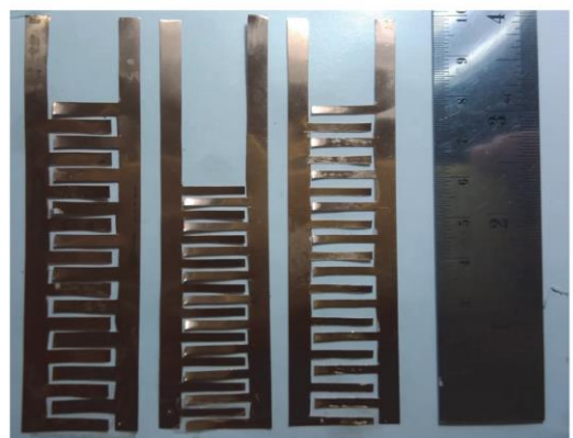
Fig.3. The fabricated IDC level sensor with non-substrate .
