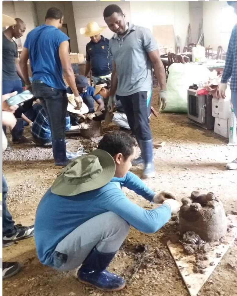
Figure 1.6 Make rocket stove with mud
