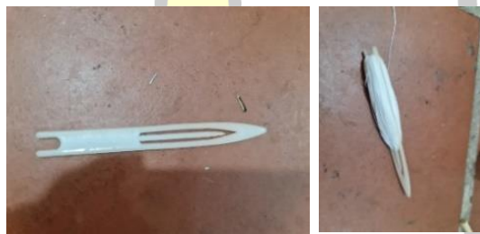
Figure 72 Tool used to wrap the threads to shape the lantern Source: Nguyen Thi Thanh Thao (May 24, 2022)
