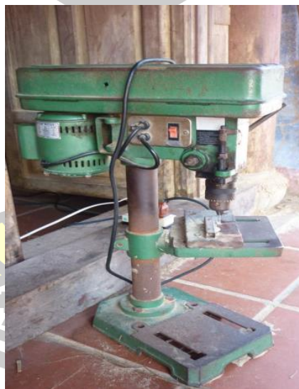
Figure 70 Hole drilling machine bamboo slats Source: Nguyen Thi Thanh Thao (May 24, 2022)
