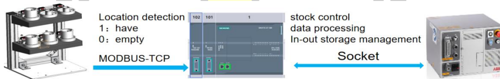
Figure 12: Device communication and connection
