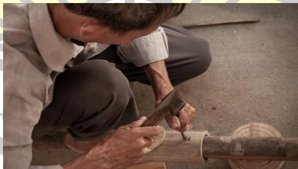
Figure 70. Treatment of the connecting part of the Goutong
