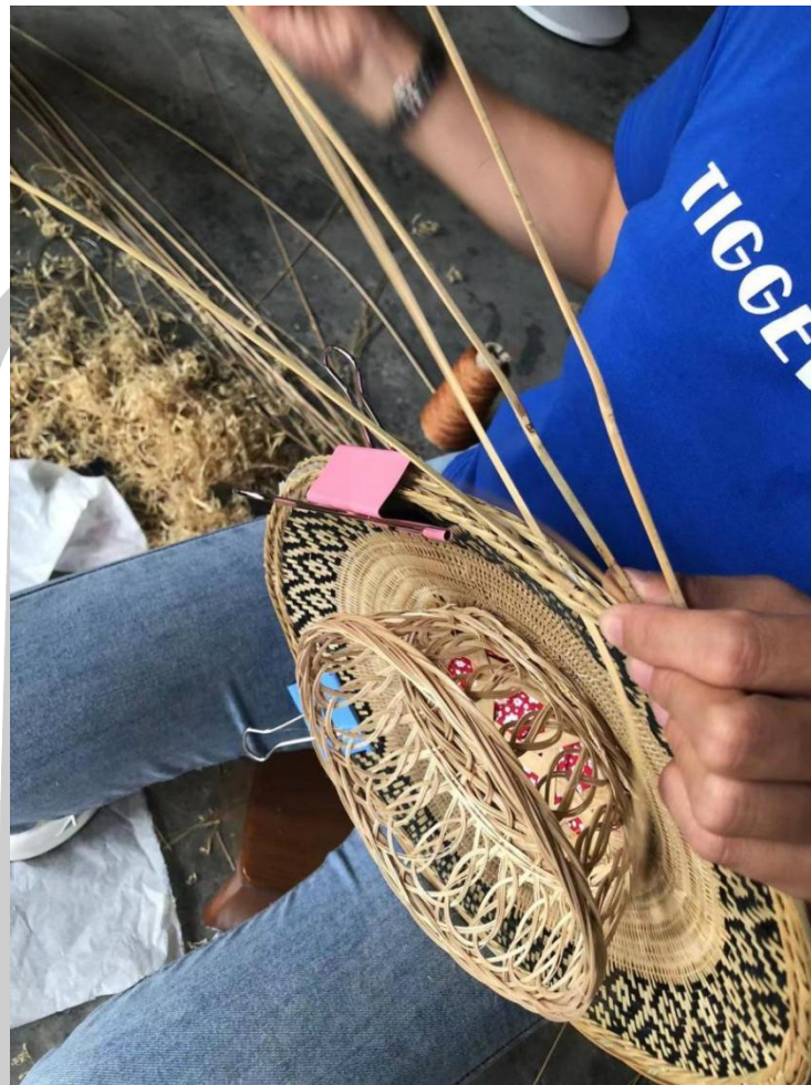
Figure 40 Flower bamboo hat body integration process (through this step, the two single pieces of the hat integrated together to become a complete a hat)
