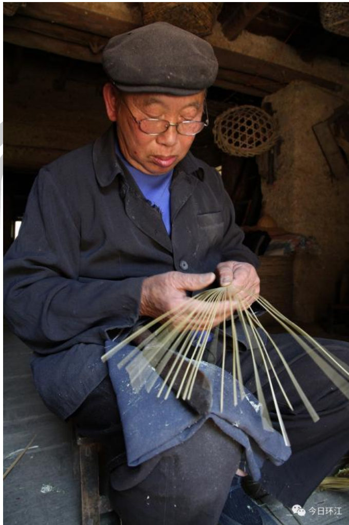
Figure 32 Tan Shunmei making bamboo strips for gabions by hand Source: Baidu Gallery, September 15, 2022
