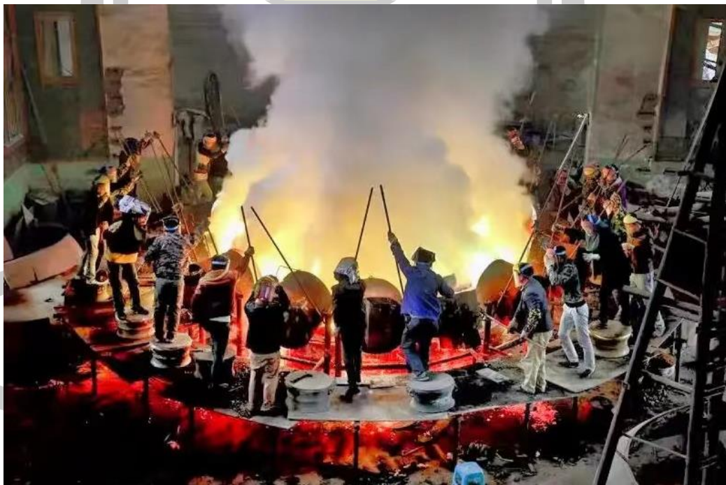
Figure 37 2017 Guinness's "the largest copper drum" We's giant copper drum making, casting site
