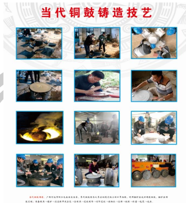
Figure 41 Contemporary copper drum casting technique flowchart Source: Yongfa Wei, February 3, 2023
