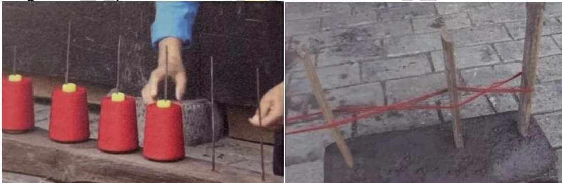
Figure 49 Place the bobbins on the warp beam
