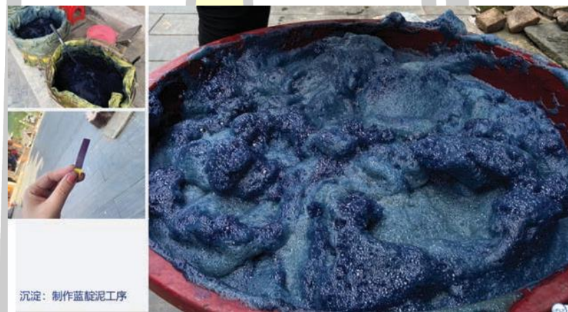
Figure 18 The purification of indigo water to create bubbles. Pour water into the bucket to allow the microorganisms in the dye tank to receive oxygen. Source: Photographed by the author. July 31, 2021
