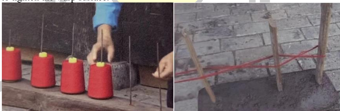
Figure 40 Place the bobbins on the warp beam Source: Photographed by Li Cheng Feng, July 20, 2018, Tujia women participate in training at the Lachahe Tujia brocade workshop
