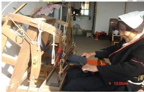
Figure 13 Women in Mentou Village are weaving brocade. There are two forms of Hualan Yao garment making techniques, embroidery and brocade weaving. The headscarves, belts and bindings of the Hualan Yao garments are woven on looms.
