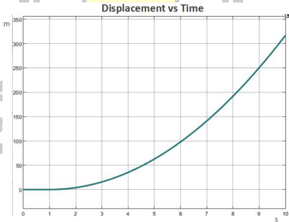
Figure 38 6x1kW-FW MATLAB-Simulation Displacement vs Time
