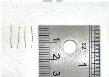
(a) Single-size steel fiber
