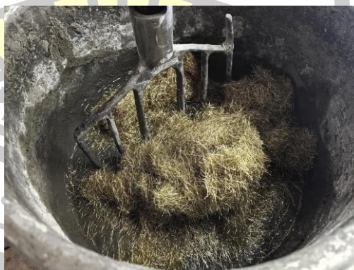
Figure 14. Adding steel fiber and continue mixing.
