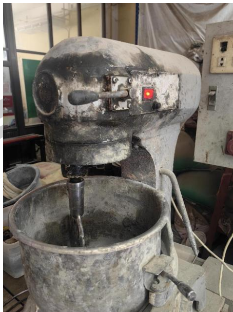
Figure 18. The 20 litre standard mixer from Bosson Ltd in Thailand.
