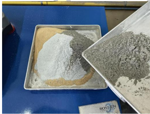
Figure 13. Mixing all binders and sand in a tray.
