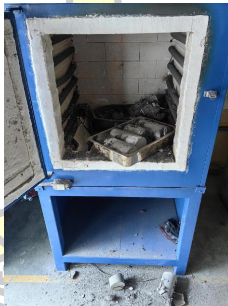
Figure 35. Explosive spalling of samples at high temperatures.
