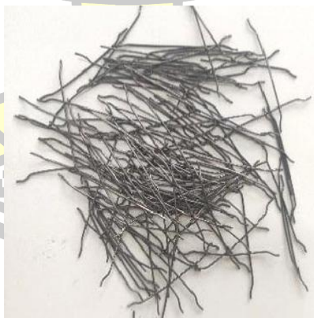
Figure 3. Hooked-end steel fiber [26] .
