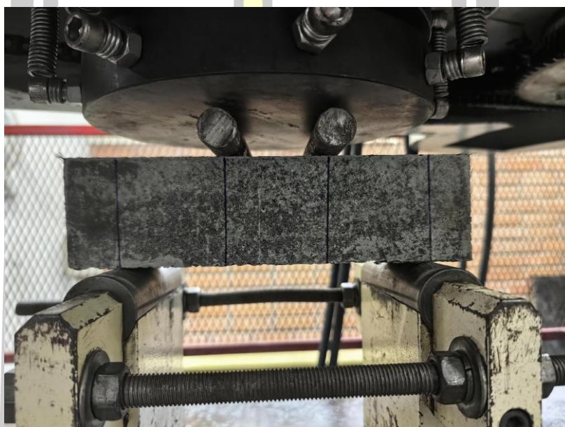
Figure 24. Flexural strength test according to ASTM C1609.
