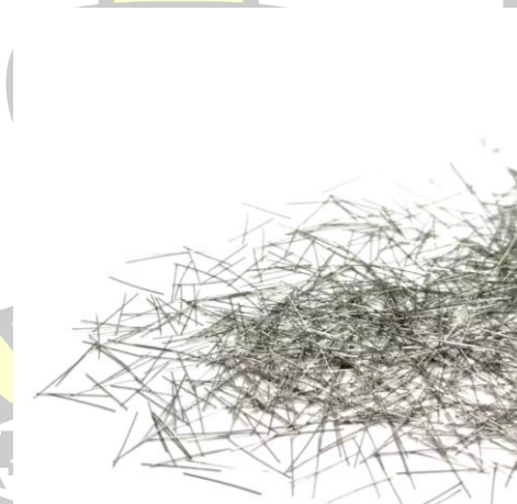
Figure 5. Straight steel fiber [27].
