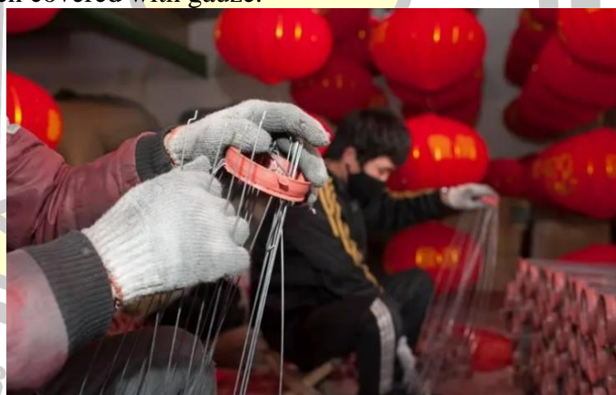
Figure 45 Modern red gauze lanterns with steel wire skeleton and plastic upper and lower seats
