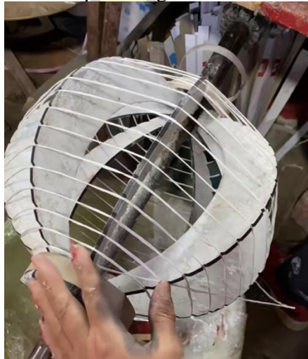
Figure 69 Semi-mechanized production of red yarn lantern skeleton source: https://image.baidu.com/baike
