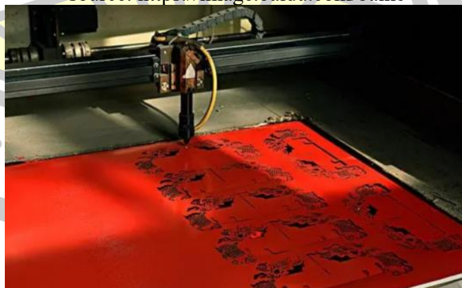
Figure 70 Laser engraving craft paper lanterns source: https://image.baidu.com/baike
