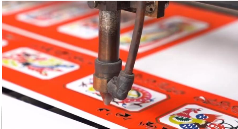
Figure 37 Laser engraving of the openwork decoration of the lantern frame Source: Wang Kun, May 6, 2023, Ligaocheng Palace Lantern Museum, Shijiazhuang, Hebei, China
