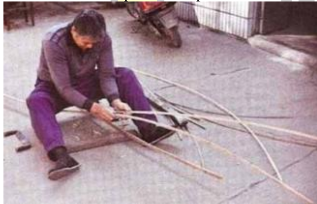
Figure 22 Splitting bamboo strips in the process of making a traditional lantern Source: Courtesy of Li Na (staff member of the Ligaocheng Palace Lantern Museum), Ligaocheng Palace Lantern Museum, May 6, 2023
