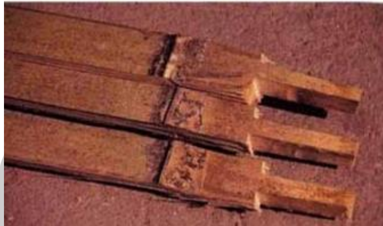
Figure 23 Cutting the head during the production of a sarong lantern Source: Courtesy of Li Na (staff member of Ligaocheng Palace Lantern Museum), May 6, 2023, Ligaocheng Palace Lantern Museum
