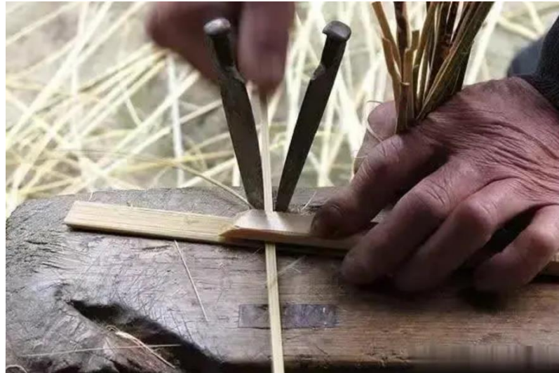
Figure 68 A lantern craftsman digging bamboo gabions by hand Source: https://image.baidu.com/baike
