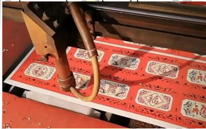
Figure 32 Ligucheng Craft Paper Lantern Laser Engraving
