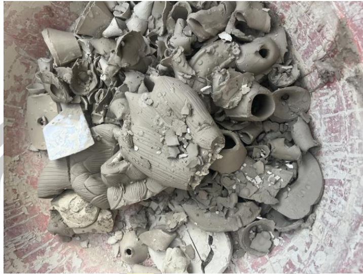
Figure 134.Failure due to improper moisture adjustment Source: Photography by Zhang Lin, 2023
