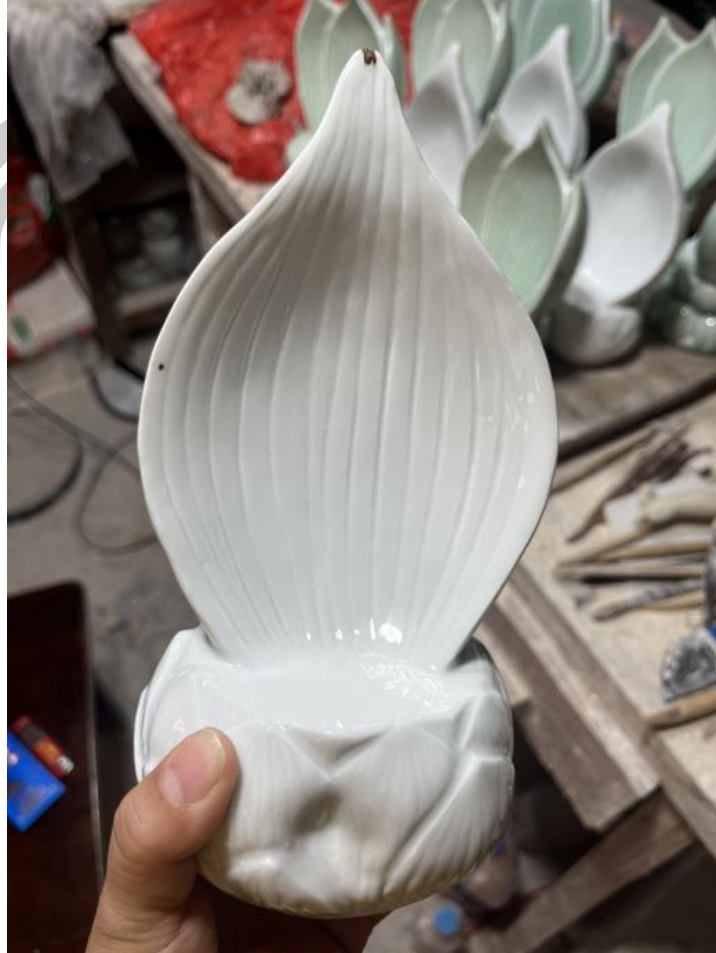
Figure 136. Blackening of the top due to not applying zinc water to the top during firing
