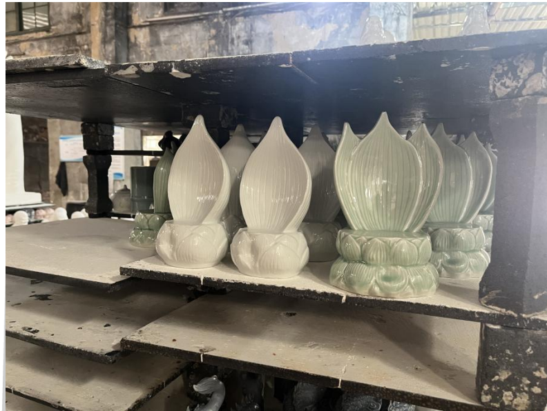
Figure 129 The intake kiln is fired at 1300 degrees Celsius Source: Photography by Zhang Lin, 2023
