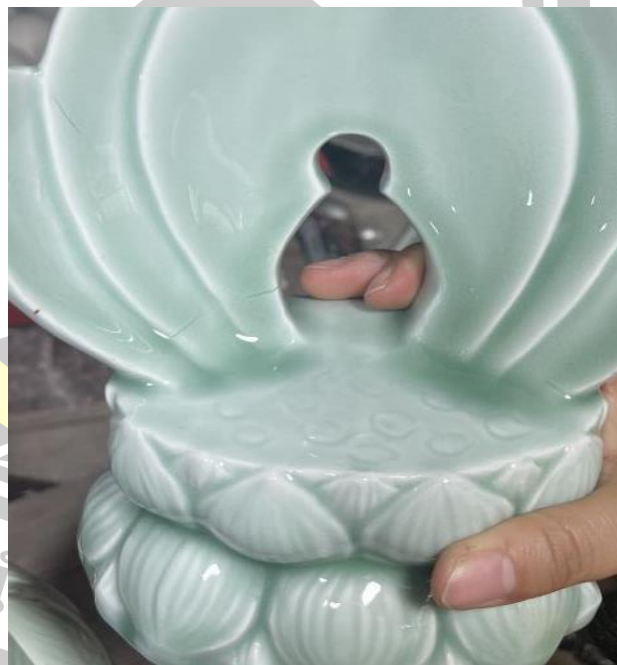
Figure 135.Glaze cracks due to uneven temperature of kiln fire Source: Photography by Zhang Lin, 2023
