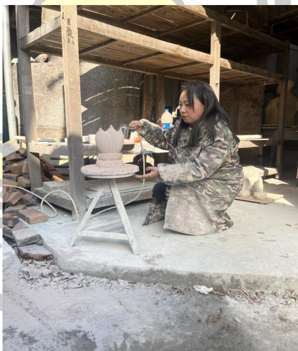
Figure 128. Glaze with a watering can Source: Photography by Zhang Lin, 2023
