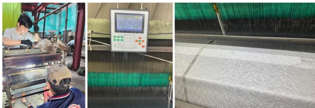
Figure 43 Quang Nam weavers improve tools to increase silk-weaving productivity. Quang Nam weavers have researched and applied CNC programming technology in wood and industrial iron carving to replace the traditional punched card weaving method. This new approach can weave patterned silk fabrics up to 1.8 meters wide, allowing for the simultaneous weaving of seven colored threads.
