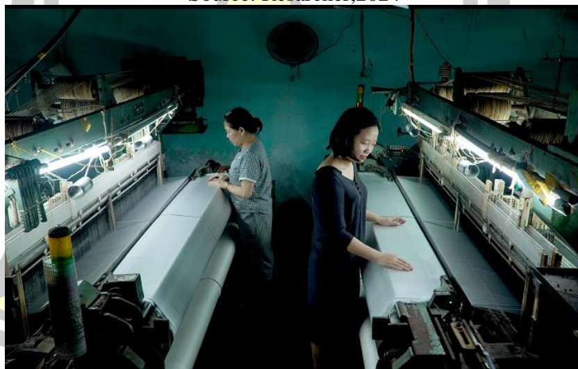
Figure 42 The modern looms in Quang Nam. The modern machiner helped Quang Nam weavers to weave silk sheets of much larger sizes than before.
