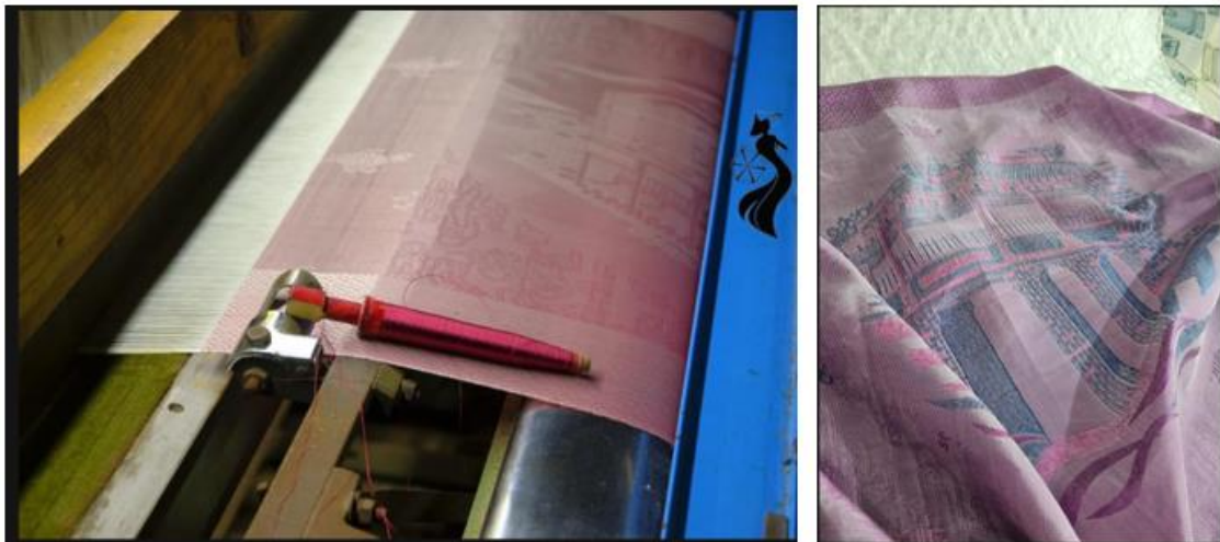
Figure 68 Patterned Gam Silk weaving. The successful modification of the gam weaving machine is a significant milestone in the revival of the silk weaving craft. As of September 2023, Ma Chau is the first production facility in Vietnam to have successfully improved the gam weaving machine. Besides helping manufacturers shorten weaving time, this machine can also weave various large-sized patterns, something traditional weaving machines could not achieve
