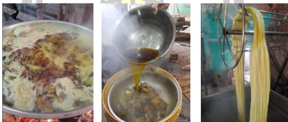
Figure 44 Fibraurea tinctorial dyeing process In reality, achieving color accuracy with natural dyeing is challenging. Even a slight change in the dye solution's concentration, temperature alterations, dyeing time, or the addition or subtraction of other additives can significantly affect the intensity of the color in the finished silk product.
