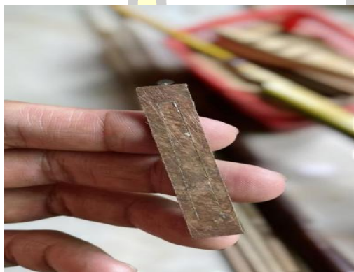
Figure 30. Cutting copper reed
