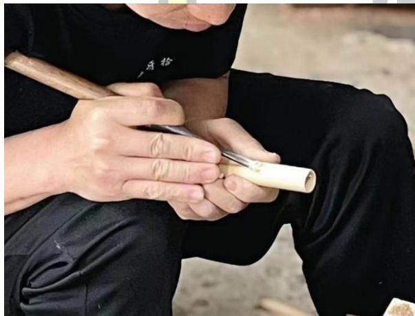
Figure 34. Grooving of sound pipes
