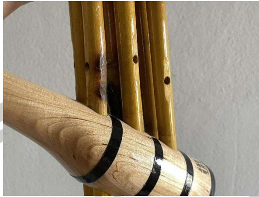
Figure 35. Drill sound hole
