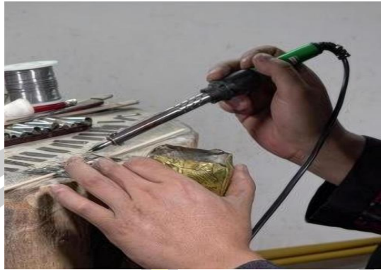
Figure 31. Adjusting the pitch of the reed
