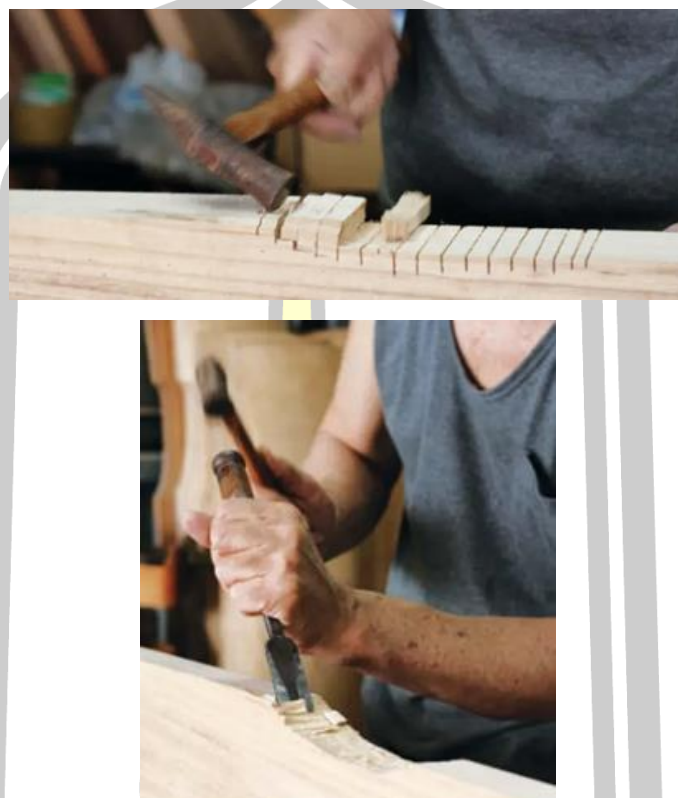
Figure 6. 26 Waist way of making Guqin
