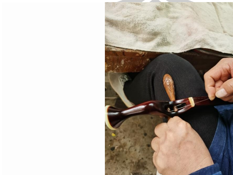
Figure 27. The strings need to be threaded through the tuner holes
