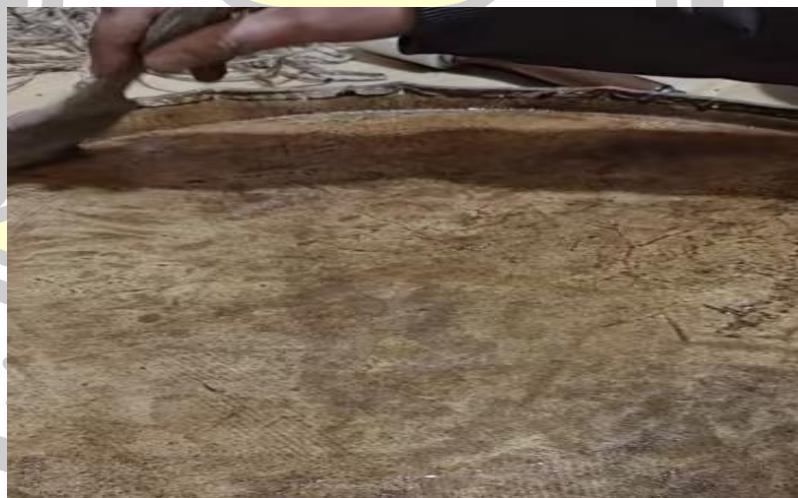
Figure 28. Brush hardened latex to increase the hardness of dry drum
