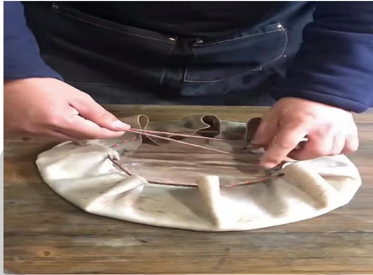
Figure 27. Secure and tighten the drum cover
