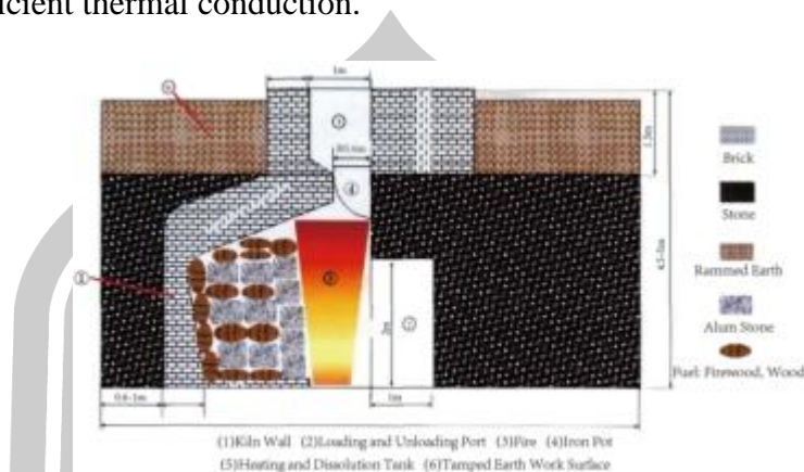
Figure 20: Second-Generation Crucible Roasting Furnace
