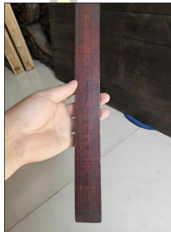
Figure 33 Luban ruler made by Mr. Yang Yundong, a Dong carpenter. The words marked above represent lucky or unlucky dimensions. Dong craftsmen use special Luban rulers to choose lucky sizes to build houses, bridges and so on. Source: Photographed by Yang Yundong. December 1, 2023
