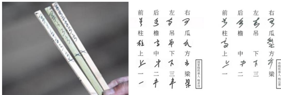
Figure 39 "Moshi" Character. The unique architectural symbol "Moshi" Character of the Dong people. They are carved on the "Jianggan" and on building components to help Dong craftsmen mark the building component and its orientation. Source: Photographed by Chen Lu. November 3, 2023
