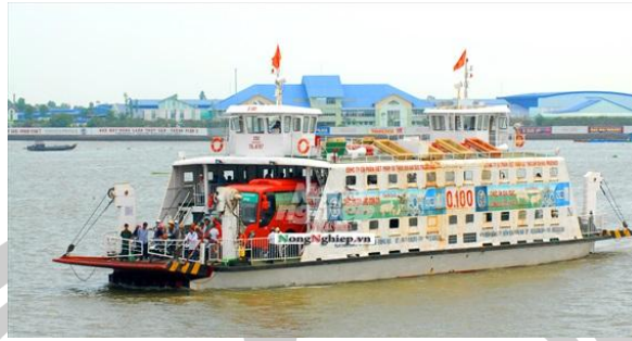
Figure 77 Ferries are large in size and capacity and are used to transport passengers and vehicles on large rivers. The ferry has two ends for convenient docking on both sides of the river.
