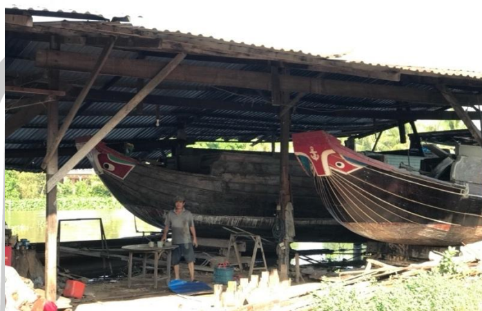
Figure 231. The big boat on the viewer's left is Ghe Bau - Ghe Tam Ban Can Tho. Can Tho boats have a large body, the belly of the ship is big, but the boat's bow is slim, and the body behind the rudder is also relatively slim, mainly moving on calm water, the current is not too strong.
