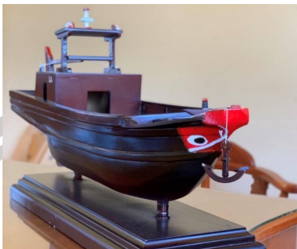
Figure 106 Ghe Cui Can Duoc: The boat has a slightly rounded bow without a horizontal slat, formerly known as a pig's beak.
