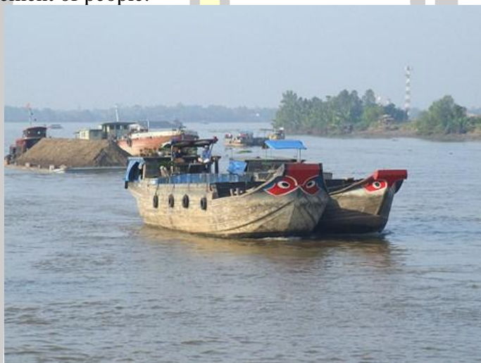
Figure 228 The big boat on the viewer's left is Ghe Bau - Ghe Tam Ban Can Tho. Can Tho boats have a large body, the belly of the ship is big, but the boat's bow is slim, and the body behind the rudder is also relatively slim, mainly moving on calm water, the current is not too strong.
