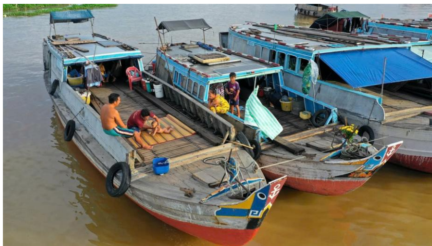
Figure 229. When Ca Dom boats want to transport fresh fish, they create a water vent under the boat's hold to become Duc boats. Otherwise, they still create the shape of Ca Dom boats to transport goods normally..
