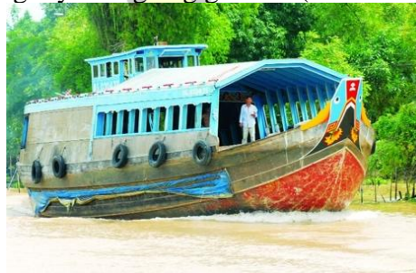
Figure 66 “Ghe Duc” Duc boat is moving on the river after releasing water from the fresh fish tank, it will float up high.
