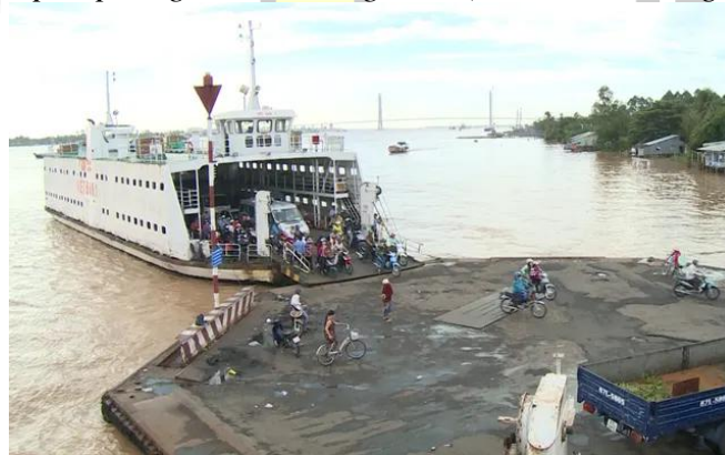
Figure 75 Ferries are large in size and capacity and are used to transport passengers and vehicles on large rivers. The ferry has two ends for convenient docking on both sides of the river.
