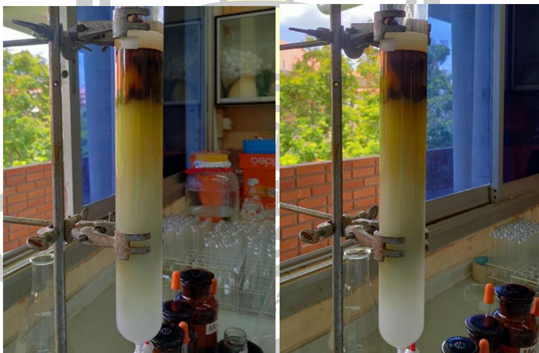
Figure 8. The isolation of the EtOAc extract of G. vidalii by column chromatography.
