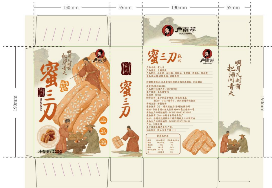
Figure 58 Aircraft box structure dimensions Source: Drawn by the author(2024)
