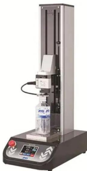
Figure 10 MCT-1150 tensile machine. AiAnde. Japan
