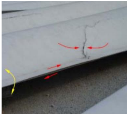
(a) Blade Cracking
