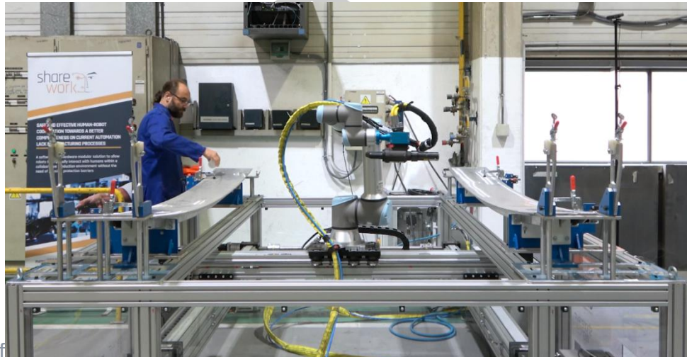
Figures 4 Human and robot corporate in tramway sub-assembly processes [9]
