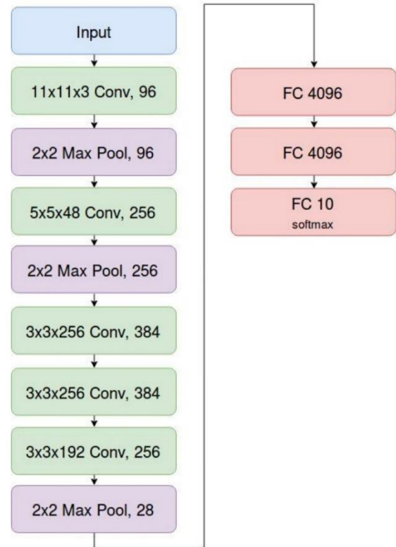
Figure 4 The AlexNet architecture.
