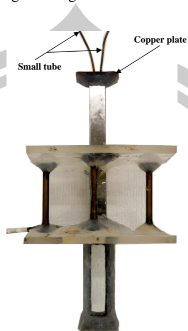
Figure 3.3 The rectangular cross sectional pipe with installation Copper plate and small tubes.
